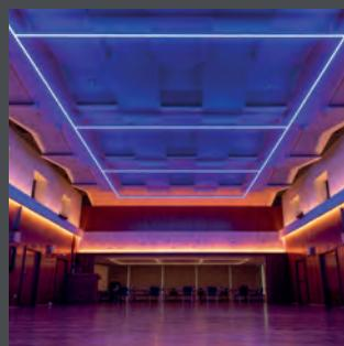
The intelligent RGBW light source consists of four different colour LEDs to achieve excellent white colour fidelity in addition to the many colours that can be chosen via DALI DT8 (Primary N).
